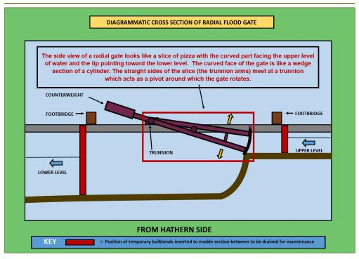
have noticed that the emergency mooring upstream of the radial gate has undergone extensive restoration for the first time since its installation. Repainting the steelwork and replacing the wooden elements of the mooring are relatively straightforward tasks compared to those involved in the servicing of a radial gate, however, and that brings us — at last — to the 'building' referred to at the beginning of this article and to an explanation of its purpose.
